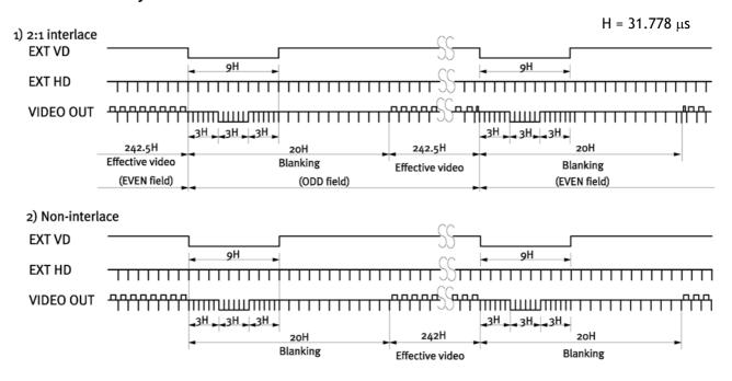
Fig. 10. Vertical timing with external sync
